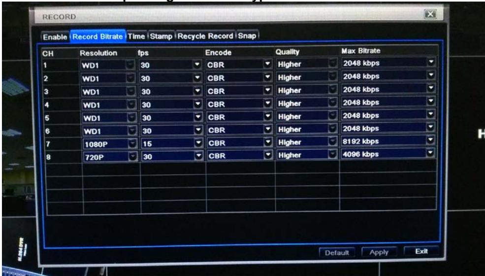
**Note:** if the rate value set is over high the maximum resources of the device, the value will be adjusted automatically.
