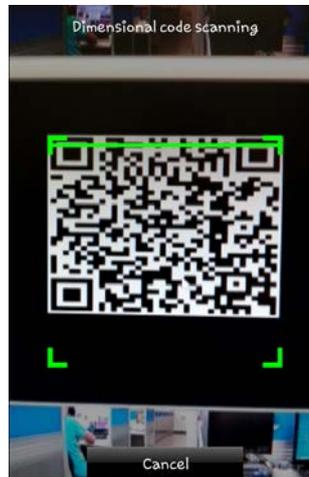
3. After finished the scanning procedure, it will automatically bring out the device MAC number and user account, user just need to key-in the password.
