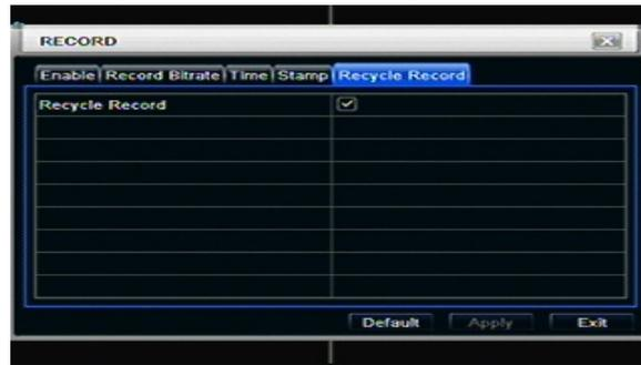
Step2: tick off recycle record, the recycle record function will enable, it will cover the earlier recorded files and keep recording when HDD is full; if disenable this function, it will stop recording when HDD is full.
