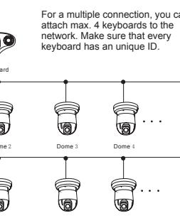
For a multiple connection, you can attach max. 4 keyboards to the network. Make sure that every keyboard has an unique ID.
