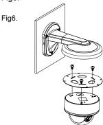
Mount the dome camera (with the metal plate) to the top plate of the bracket by 4 screws shown as Fig7.
