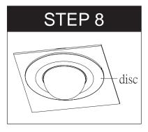
Rotate disc in the direction shown in this picture to hold metal plate
