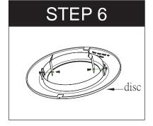
Use 2 screws and 2 screw bolts to fix 2 metal pieces onto the disc
