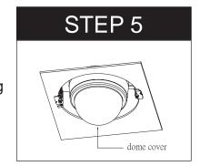
After camera is properly adjusted, put on dome cover by rotating in the direction
