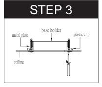
Then use screwdriver (counter-clockwise) to fasten base holder on ceiling
