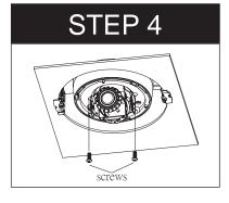
Use 2 pcs screws to fix dome camera on metal plate of base holder
